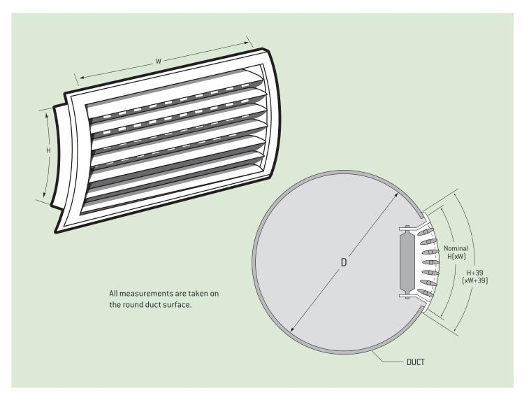
The TLC version of certain sizes of models DDL & SDL20 has been specifically designed for direct mounting on to Holyoake Spiroloc rigid round duct. Only the heights listed are available and only the units with front blades in the 'W' direction (DDL and SDL) can be produced.
