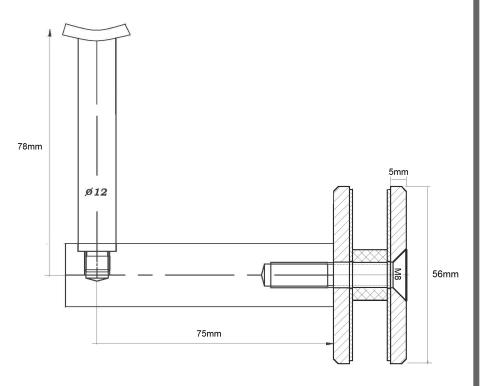
Visible 8mm countersunk screw fixing
