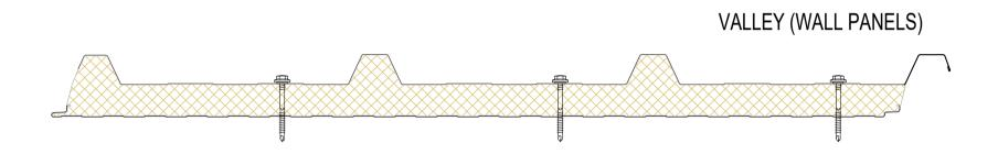
KS1000 RW WALL PANEL <u>PRIMARY FIXING LOCATIONS</u>. HORIZONTALLY OR VERTICALLY LAID
