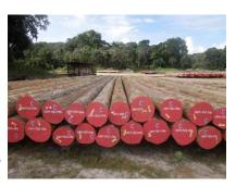
**Mechanical properties:-** Has exceptionally high strength properties even when its weight is taken into account. Weight about 1030kg/m3 (64lb/ft3) seasoned. Bending strength 181 N/mm2 (26200 lbg/in2). Compression parallel to grain 89.9 N/mm2 (3040 lbg/in2)
