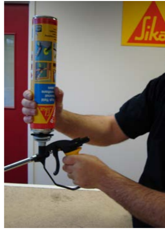
With the can facing away from your body, screw the can onto the Sika Boom-G Gun. Make sure the can is "hand tight". You may hear a hiss as the can attaches to the adaptor.
