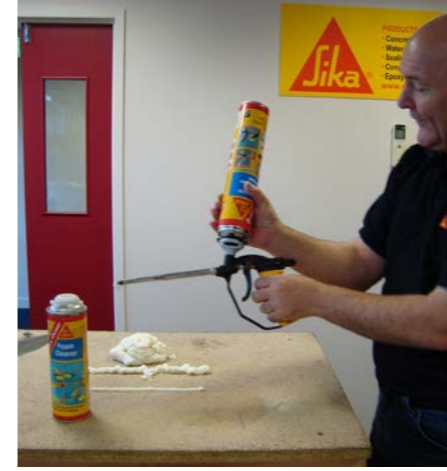
Hold the can away from your body, unscrew the can from the dispenser gun.
