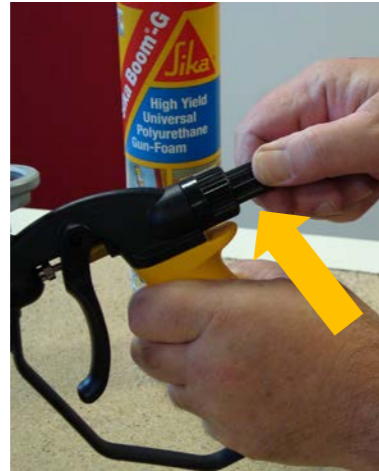
Make sure the valve regulator is turned off by turning it clockwise.
