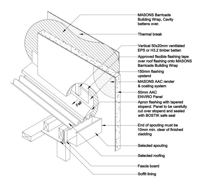
**ROOF/WALL JUNCTION -**KICKOUT FLASHING
