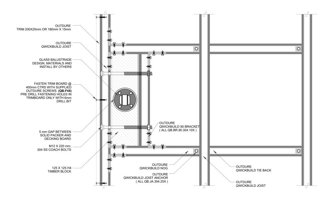
QB-G3. BALUSTRADE PARALLEL TO JOIST DIRECTION FOR 90mm JOIST ( PLAN VIEW )
