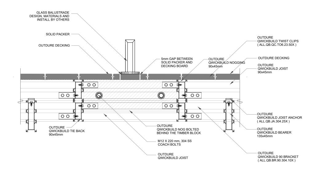
QB-G3. BALUSTRADE PARALLEL TO JOIST DIRECTION FOR 90mm JOIST ( SECTION VIEW 1)
