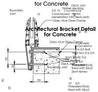
Architectural Bracket Detail for Decking Flashing Glass Vice Glass Clampywood Concrete 90mm into double boundary joists Stanc Glassviae Architec Grad Box Cold Papoil Cladding for Decking Glass Hich Glass Glamp S/S Washer Deck Joist Boundary Joist
