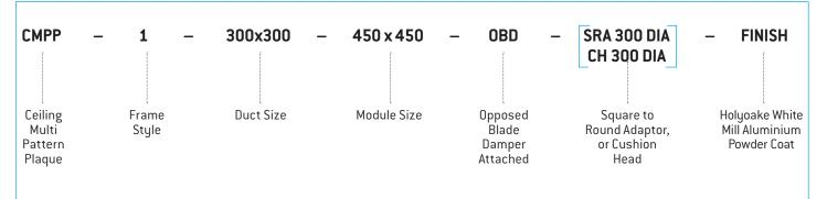
Ceiling Multi Pattern - Plaque Louver Face diffusers shall be type CMPP. They shall be of all Aluminium construction, with removeable plaque core. CMPP have a range of frame styles and accessories for installation and volume control.
