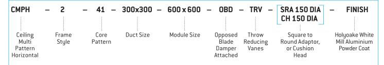
Ceiling Multi Pattern Horizontal Louver Face diffusers shall be type CMPH and be all Aluminium construction with additional horizontal blades. Complete with removeable core to give multiple air distribution patterns. They shall be available with a range of frame styles and accessories for both throw adjustment and volume control.
