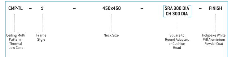
Ceiling Multi Pattern - Thermal Low Cost Louver Face diffusers shall be type CMP-TL. They shall be of Aluminium construction, with removeable cores. CMP-TL central cores, are complete with a vertical supply section controlled by a thermally actuated damper. Supply air is diffused horizontally below temperatures of 24°C and vertically with temperatures above 30°C.
