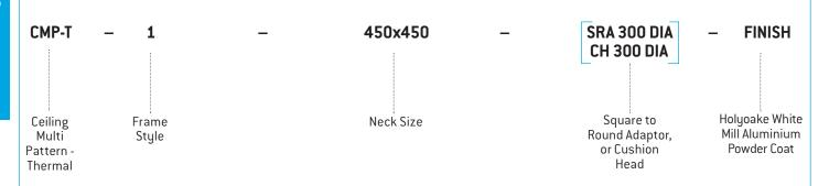
Ceiling Multi Pattern - Thermal Louver Face diffusers shall be type CMP-T. They shall be of Aluminium construction, with removeable cores. CMP-T central cores, are complete with a vertical supply section controlled by a thermally actuated damper. Supply air is diffused horizontally below temperatures of 24°C and vertically above temperatures of 28°C.
