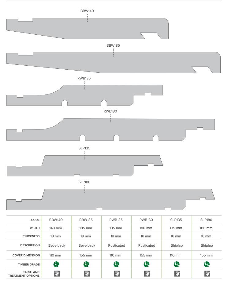
Install and fasten all weatherboards as per New Zealand Building Code. For more detailed instructions on weatherboards refer to www.smartclad.co.nz or the Purepine Smartclad Weatherboard brochure.
