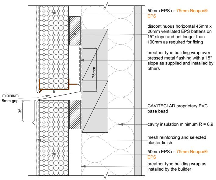
note: this detail is required at the second storey joist level. refer to NZBC E2/AS1, clause 9.1.9.4B
