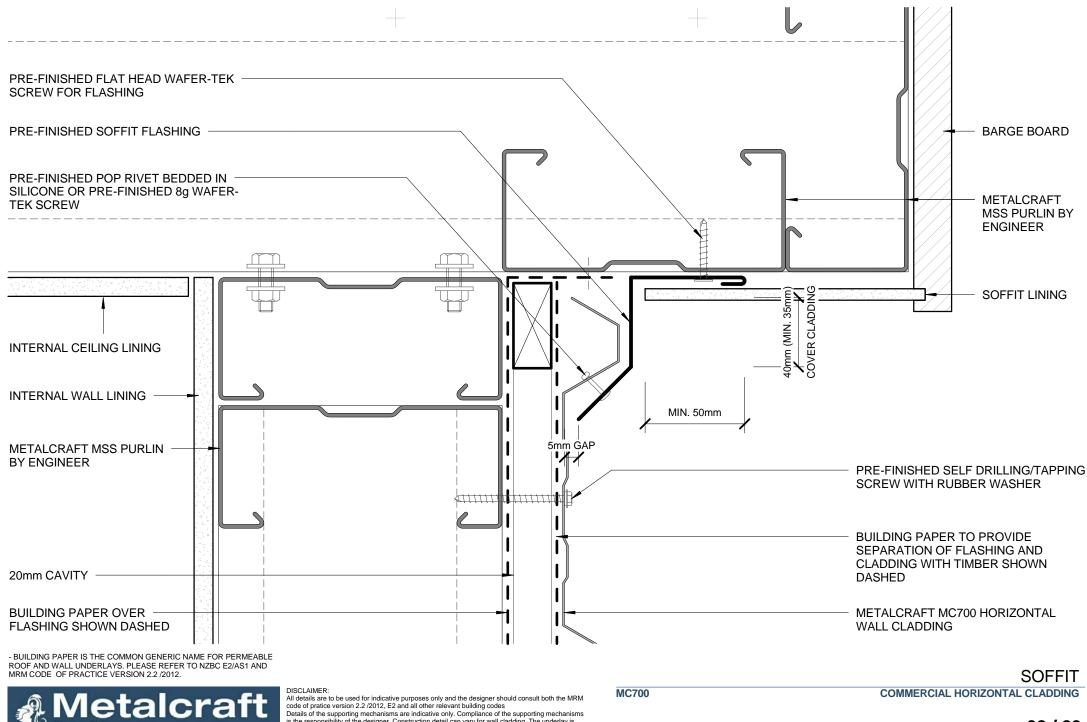
is the responsibility of the designer. Construction detail can vary for wall cladding. The underlay is detailed as a single line for simplicity and is indicative only. Building paper type and method of installation should comply with underlay manufacturers recommendations and NZBC regulations.
