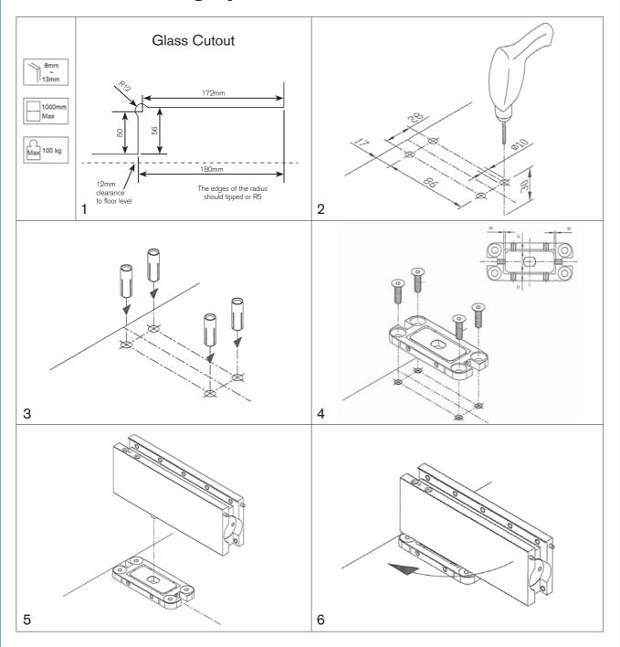
Once the patch is at 90° to the base the gaskets can be added and the door slid onto the patch and clamped in place by tightening up the screws on the side.
