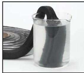
*When hydrated, WATERSTOP-RX can expand up to three times its size in an unconfined area but is limited to controlled expansion in a concrete joint where it is confined.*
