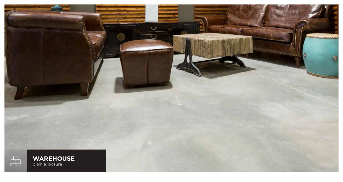
WAREHOUSE has only a resin diamond polished finish. There is no grinding of the surface laitance and no exposure of aggregates. The floor is polished to a high gloss finish following the contours of the concrete.
