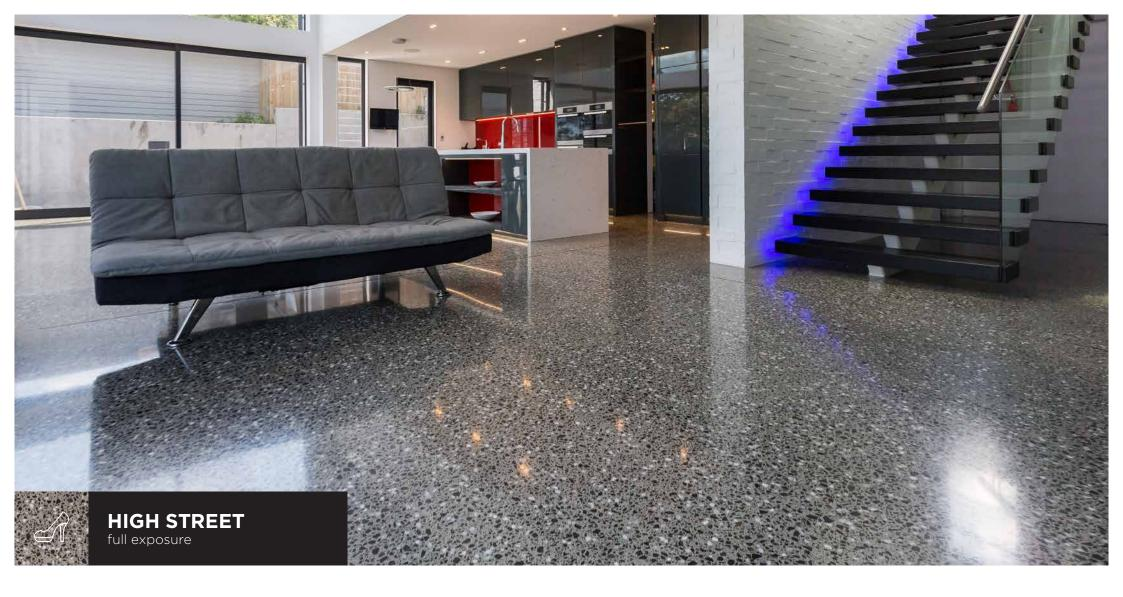
HIGH STREET is the most recognisable and preferred diamond polished finish. The process requires the removal of 3-5mm of the concrete laitance to reveal the underlying aggregates. The floor is ground flat leaving a mixture of heavy stone and fine aggregates that are then resin diamond polished. The floor is created using well established megafloor processes with internationally recognised and quality assured, equipment, tooling and chemicals.
