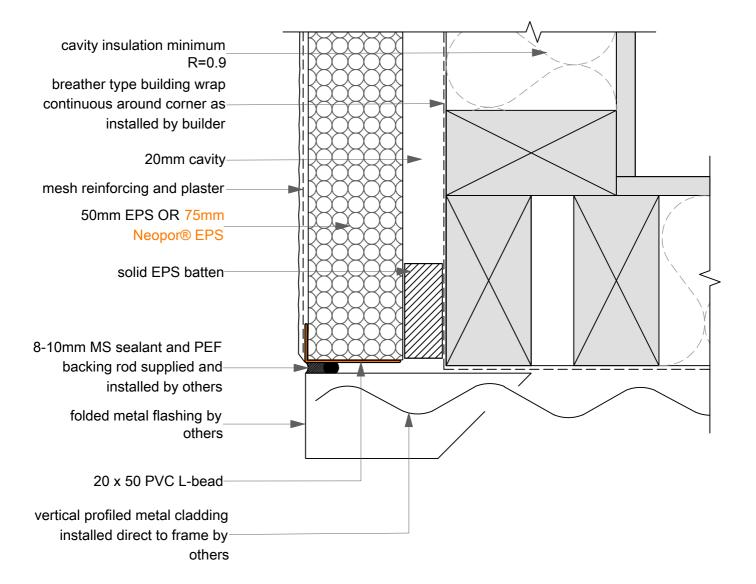
04I Wall: External Corner - PROFILED METAL SCALE: 1:2 CAVITECLAD
