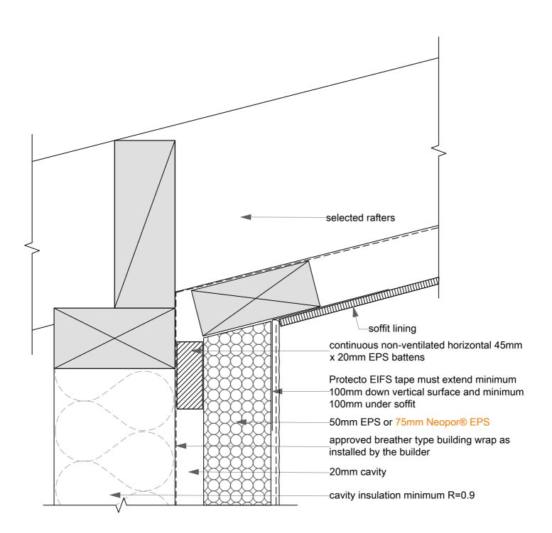
**16D** Wall / Roof: Raking Soffit (Hidden Flashing) SCALE: 1:2 CAVITECLAD
