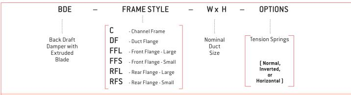
Back Draft Dampers shall be constructed from extruded aluminium.
