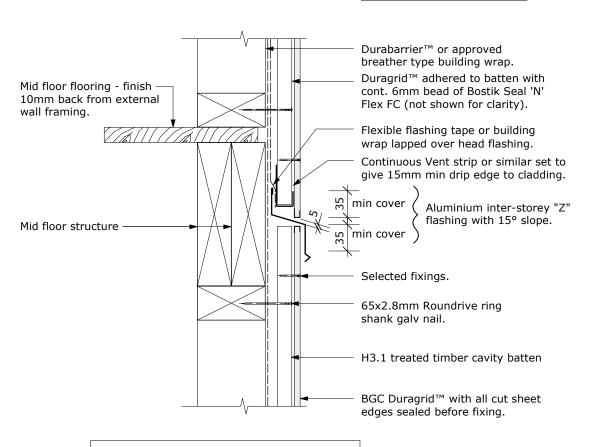
Note: Drained joints must be used to limit cavities to maximum 2 storeys or 7m in height in accordance with NZBC acceptable solution E2/AS1 Paragraph 9.1.9.4
