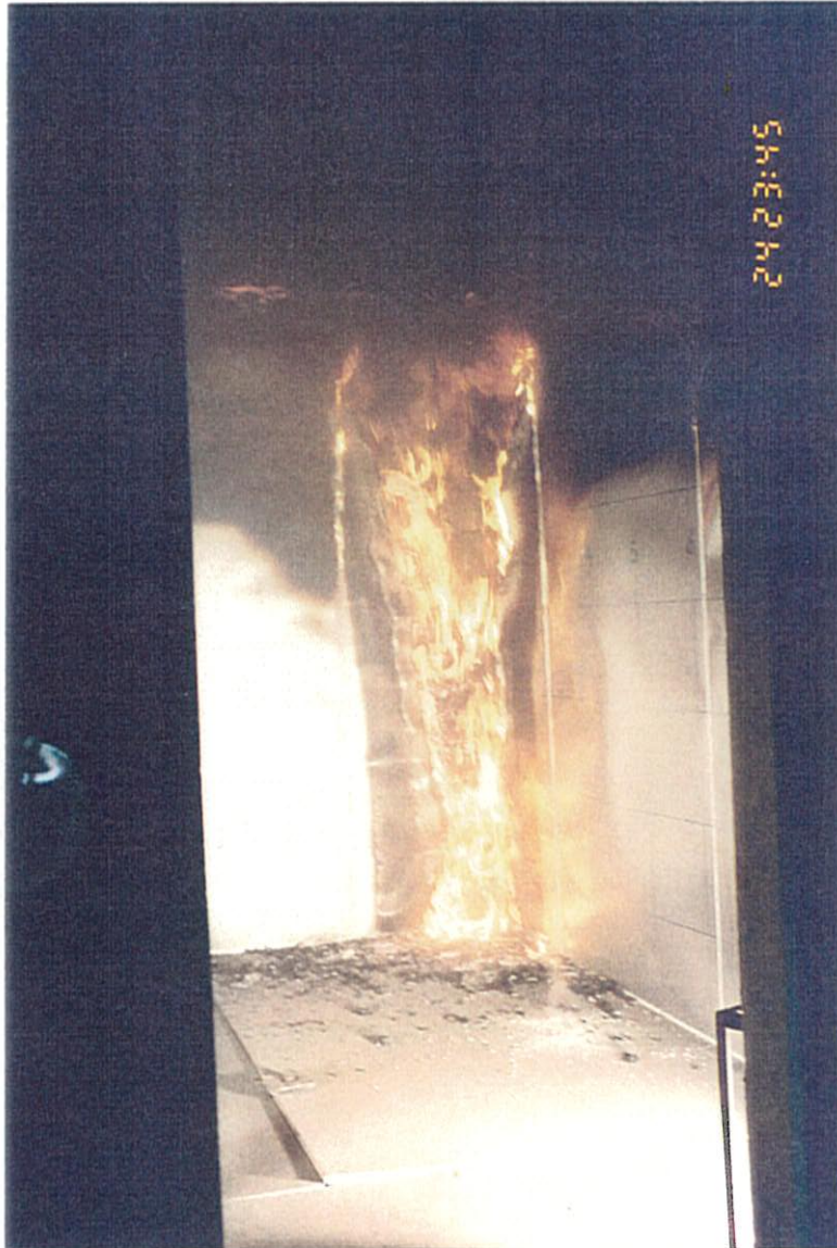
Figure C-2. Burner Corner Section at the End of 300-kW Exposure.
