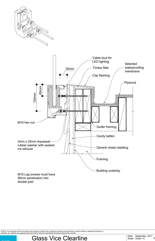
Panel Mounted Fixing Detail - 4 Point
