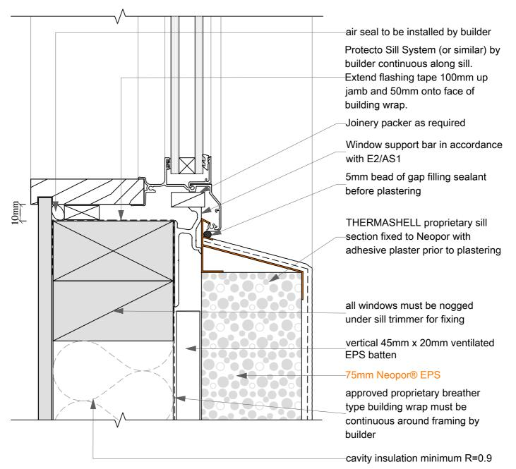
caution: to ensure the proprietary flashings for this system can be installed correctly, please allow a gap of 24mm from the surface of the building paper to the backside of the aluminium joinery note: a 5° sloped sill trimmer must be used if the back of the glazing pocket is positioned back past the line of wall frame
