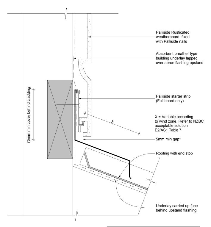
\*This detail may be used for roofs with a pitch of 12degrees minimum. Where the pitch is less than 12degrees 35mm min clearance is required between the underside of the cladding and the apron flashing
