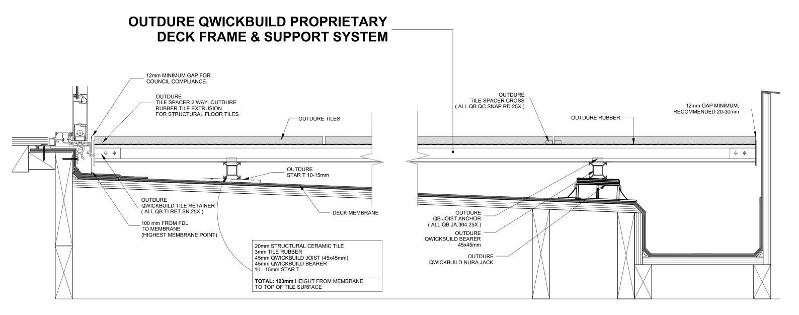
QB -T2. 100mm LOW HEIGHT TILE DETAIL SCALE 1:5
