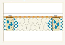
Building materials that are installed damp or that become wet or damp during construction have to be able to dry out without damaging the structure. The amount of moisture this involves is often underestimated.
