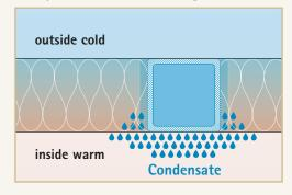
Thermal bridges contribute significantly to the growth of mould on the surfaces of building materials and to a reduction in energy efficiency.
