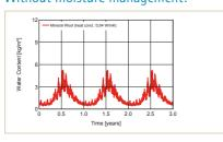
Moisture content of the 5 mm outer layer of thermal insulation rose to 5.5 kg/m<sup>3</sup>
