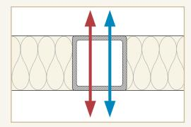
A steel support conducts the heat out of the building faster than the insulated compartment.
