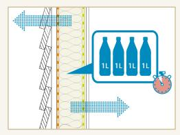
Four litres of water are added into the construction.
