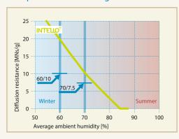
Adhering to the 60/10 rule and Hydrosafe™-value ensures a high potential freedom from structural damage for thermal insulation in new buildings and during construction.
