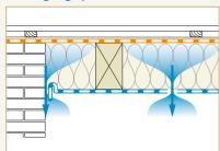
Non-airtight connection, the airtight building envelope is not continous and closed
