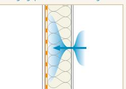
A significant amount of moisture can penetrate the building envelope by convection. This poses the risk of structural damage and mould if there is insufficient moisture compensation. The ideal solution is intelligent moisture management.
