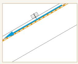
To ensure a watertight roof, at least counter battens should be used (battens along the rafters). Additional protection is provided by nail sealing tapes such as TESCON® NAIDECK under the counter battens.
