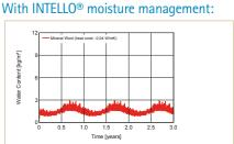
Insignificant increase in the moisture content of the 5 mm inner layer of thermal insulation
