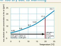
1 m<sup>3</sup> of air at 0°C and 80% relative humidity is heated to 20°C.
