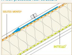
If there are rooms immediately under pitched roofs, the physical demands are similar to those for walls. The requirements for a well protected roof construction are therefore also similar to those for walls:
