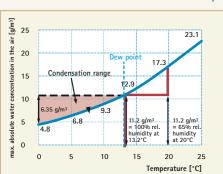
At an elevated relative humidity of 65% the dew point is already reached at 13.2°C. If the temperature drops to 0°C, significantly more condensation is deposited: 6.35 g/m<sup>3</sup>.
