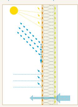
Wall wrap needs to protect the construction against the elements. It should, therefore, be:
