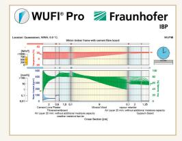
Computer-assisted simulation programme for heat and humidity transport (dynamic)
