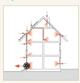
A fan creates low pressure in the building. Where there are penetrates, air enters the building from outside. These defects can then be put right relatively effortlessly.
