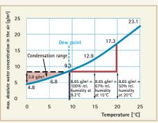
Under standard environmental conditions (20°C/50% relative humidity) the dew point is reached at 9.3°C. If the temperature drops to 0°C, 3.8 g/m³ of condensation is deposited.
