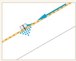
If roof battens are right on the roof underlay, the batten can act as a dam, resulting in ponding water that can then penerate around the nails.
