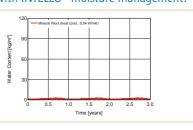
Insignificant increase in the moisture content of the 5 mm outer layer of thermal insulation
