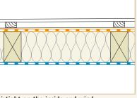
airtight on the inside and windand weathertight on the outside
