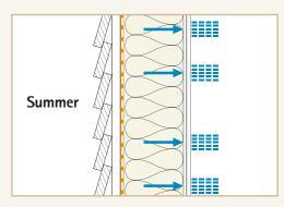
For constructions that are diffusion-inhibiting on the outside it is advisable to avoid diffusion-inhibiting material on the inside.
