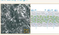
Microscopic detail of a porous membrane
