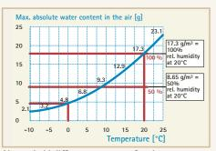
Air can hold different amounts of moisture, depending on its temperature.
