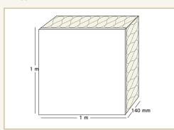
At a MVT-rate of 150 MNs/q Moisture transport in winter due to diffusion: 0.5 g/m<sup>2</sup> x 24 h
