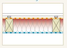
Airtight and windtight roof construction prevents heat flow by convection
