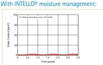
Insignificant increase in the moisture content of the 5 mm inner layer of thermal insulation
