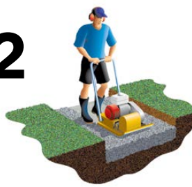
PREPARE THE BASE COURSE
