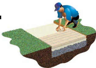
LAY THE PAVERS
