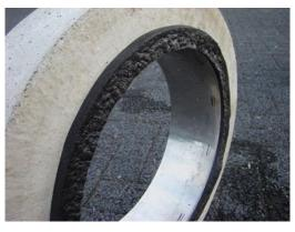
Photo 3: Indentations in soft foam from being placed on the paver surface to form a seal.
