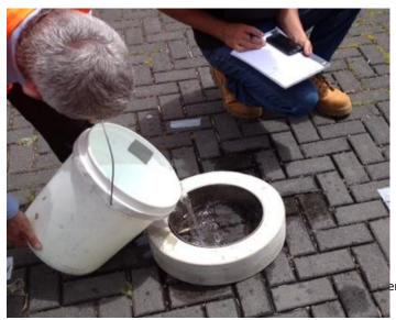
Photo 1: Timing a set volume of water, at a constant depth of 10 to 15mm, to infiltrate the pervious surface within the steel ring. Concrete surround (with a soft closed cell foam on its base, see photos 2 and 3) provides a seal to
