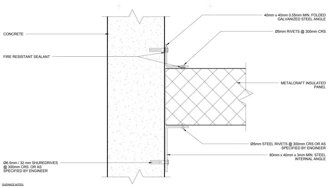
1. WHEN STANDARD INSTALLATION OF PANELS IS SUFFICIENT THEN THE STEEL FLASHINGS CAN BE REPLACED WITH ALUMINIUM
