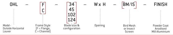
Horizontal Outside Louvers shall be of extruded aluminium construction with 100 mm blades fixed at their ends with stainless steel screws into a welded aluminium frame. The bottom louver shall overlap the frame and the structure shall be designed to with stand a wind load of  $95 \, \text{Kg/m}^2$ .
