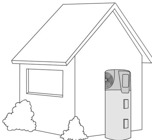
The water heater must be installed with a clearance of at least 25 mm from a wall behind the water heater. To maintain the designed performance, air flow and air discharge from the heat pump, the minimum distances to a wall or obstruction from the water heater and measured horizontally along the wall are:
