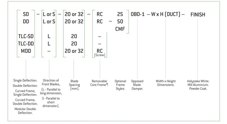
All Holyoake sidewall supply registers shall be of extruded aluminium construction, with true airfoil shaped single, or double deflection blades. Optional opposed blade volume control damper, which can be screw driver operated through the face of the grille.
