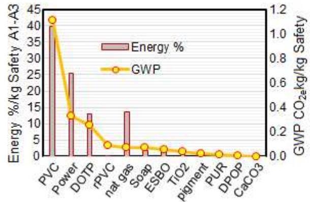
**Figure 3 Component Vs EE % share//kg A1-A3**
