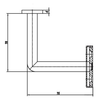
Also available without saddle for welding onto tube HBSQCP
