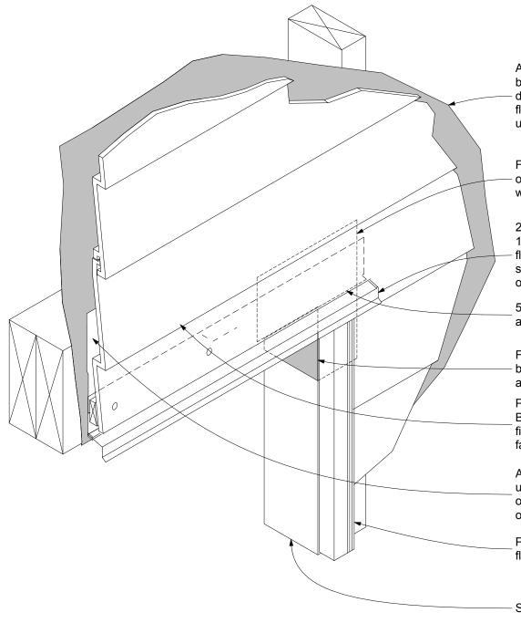
Absorbent Breather type building underlay dressed into opening with flexible tape installed over underlay to corners at head
