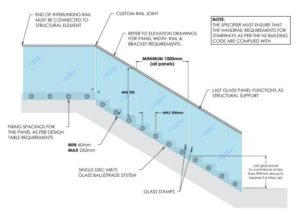
IMPORTANT NOTE: The substructure to which the balustrade is to be attached must be designed by a structural engineer to resist the relevant balustrade actions as per B1/VM1.
