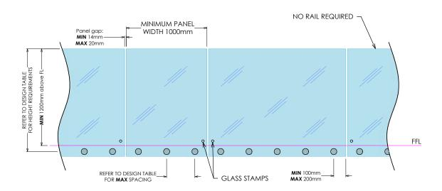
**IMPORTANT NOTE:** The substructure to which the balustrade is to be attached must be designed by a structural engineer to resist the relevant balustrade actions as per B1/VM1.
