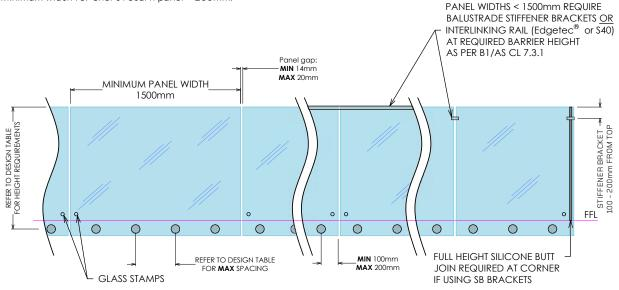
**IMPORTANT NOTE:** The substructure to which the balustrade is to be attached must be designed by a structural engineer to resist the relevant balustrade actions as per B1/VM1.
