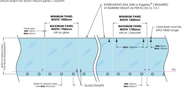
IMPORTANT NOTE: The substructure to which the balustrade is to be attached must be designed by a structural engineer to resist the relevant balustrade actions as per B1/VM1.
