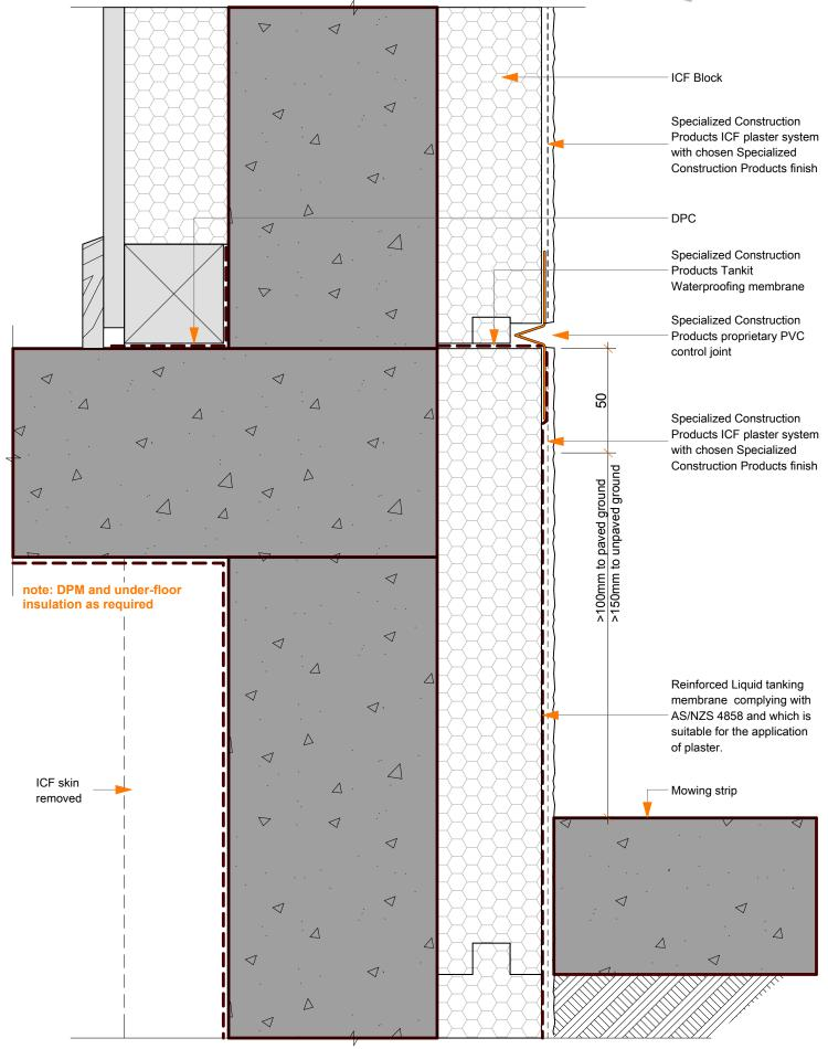
**14B** SCALE: 1:2 Wall/Floor: FOUNDATION - ICF BLOCK MLC - THIN COAT PLASTER SYSTEM
