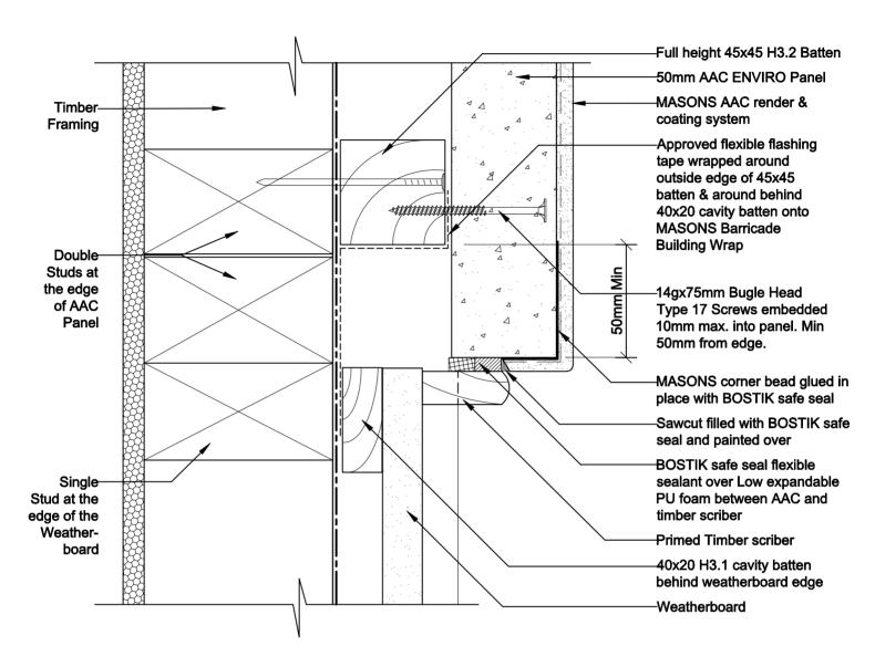
**AAC ENVIRO PANEL / WEATHER BOARD VERTICAL JUNCTION** Detail 32 Scale 1:2 **Plan View**
