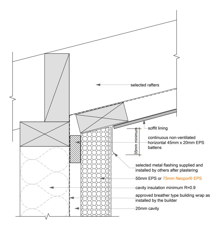
Wall / Roof: Raking Soffit (Metal Flashing)
