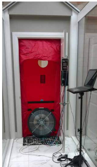
Blower door air leakage testing equipment. This is used to pressurize a building and measure how much air leaks out.
