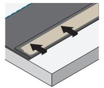
4. After flash off, fold the membrane into place then roll thoroughly.
