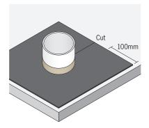
Adhere the rest of the WeldTec<sup>™</sup> membrane to overlap the base sheet beyond pipe for 100mm.
