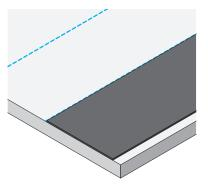
Fold back half the membrane and apply adhesive to both faces.
