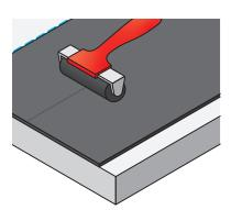
Adhere WeldTec<sup>™</sup> membrane to the floor and up the wall with a minimum cut height of 150mm.
