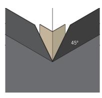
6. Cover corner point with a layer of detail tape.
