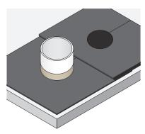
Apply collar of WeldTec<sup>™</sup> Detail Tape. Do not stretch strip. Finish with stainless steel clamp.
