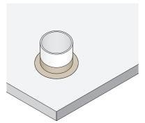
2. Adhere to WeldTec<sup>™</sup> membrane past pipe for 100mm.
