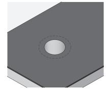
Raise the pipe through the smaller diameter hole in the WeldTec™ membrane forcing the edges upwards.
