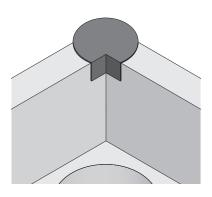
Run ARDEX Seam Tape along all four vertical sides of rainhead.
