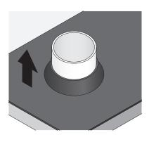
3. Pull the pipe back down 10mm to pull the membrane down and eliminate any voids.
