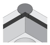
3. Cut WeldTec™ membrane to fit into corners.
