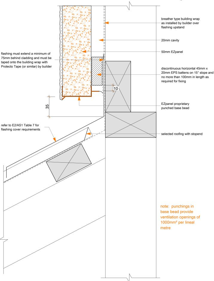
Roof / Wall: RIDGE APRON FLASHING EZPANEL
