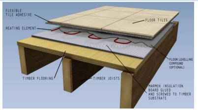
UNDERTILE HEATING WITH MARMOX INSULATION BOARD INSTALLED ON A TIMBER FLOOR.
