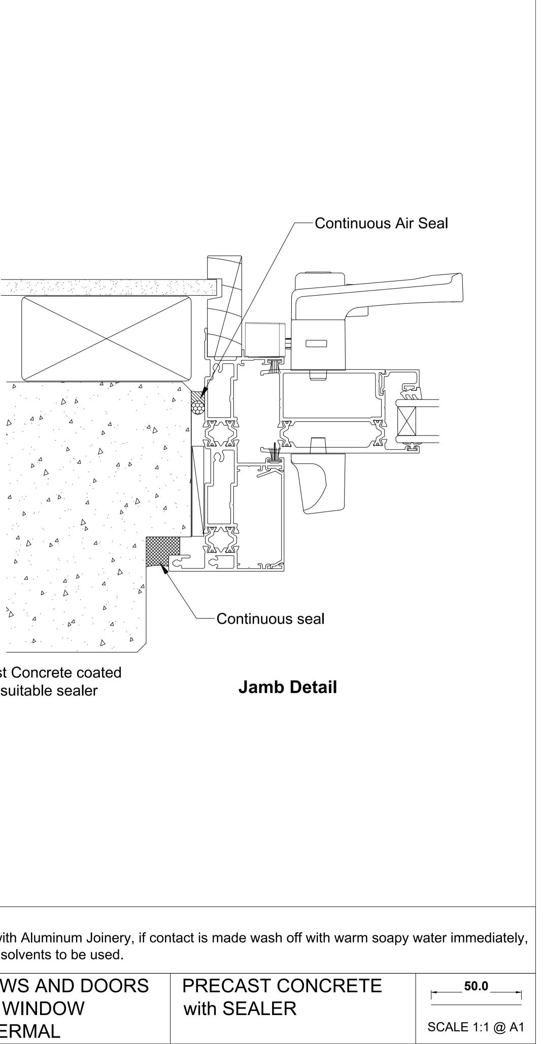
Precast Concrete coated with a suitable sealer
