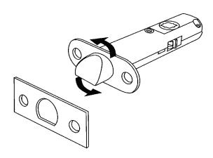
A Remove forend and rotate the latch head. Replace forend to set in place.
