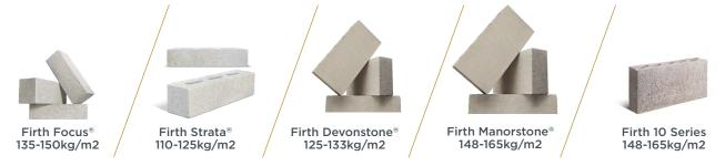
This weight is less than the maximum prescribed weight of 220kg/m² for "Heavy" claddings in NZS3604, meaning that Firth brick veneers can be used and detailed in accordance with NZS3604 for any building complying with the requirements of this document.
