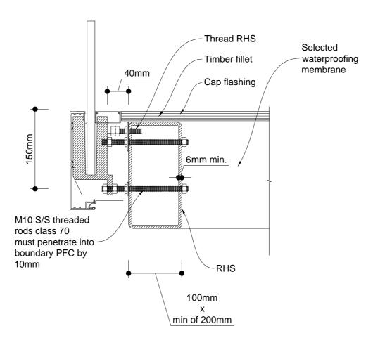
Steel members to be designed by Engineer CPEng. Spacing limited by glass capacity - refer to PS1 certificates
