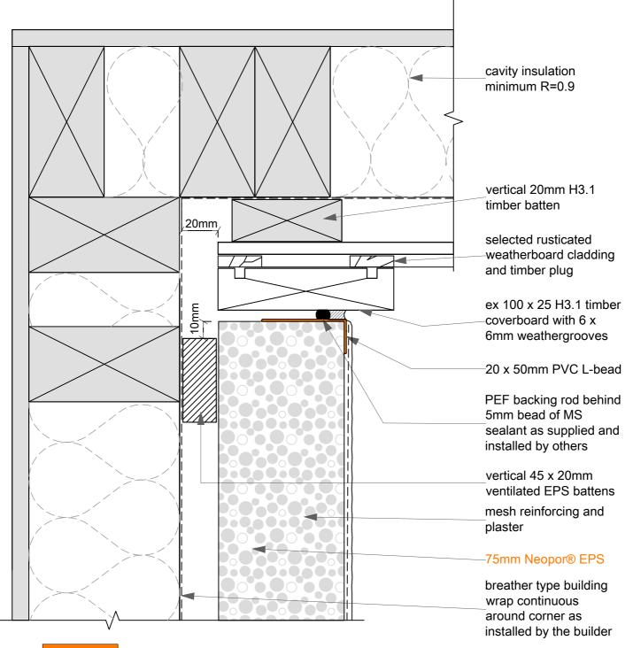
Wall: Internal Corner - RUSTICATED WEATHERBOARD THERMASHELL
