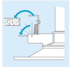
Set the trigger into the loaded position and lift the ceiling diffuser up into the ceiling opening.
