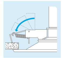
As the ceiling diffuser is lifted the trigger will activate the spring loaded holding arm to pull the diffuser up to the ceiling.
