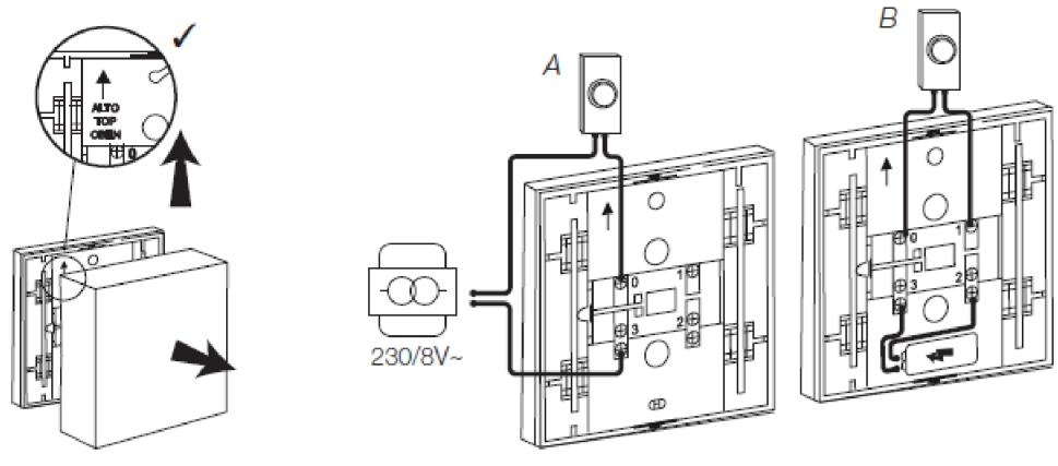
1 Lever off rear panel and screw base to wall with arrow on unit pointing UP
